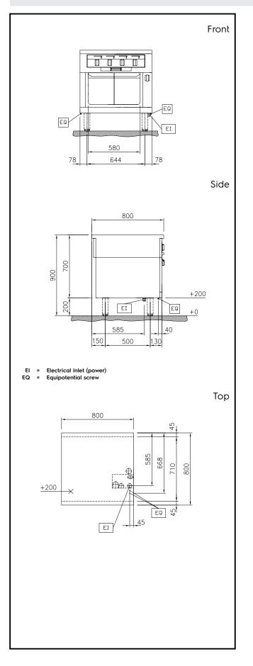
Modular Cooking Range Line thermaline 80 - 4 Zone Electric Solid Top on Warming Cabinet, 1 Side H=700 The company reserves the right to make modifications to the products without prior notice. All information correct at time of printing.
